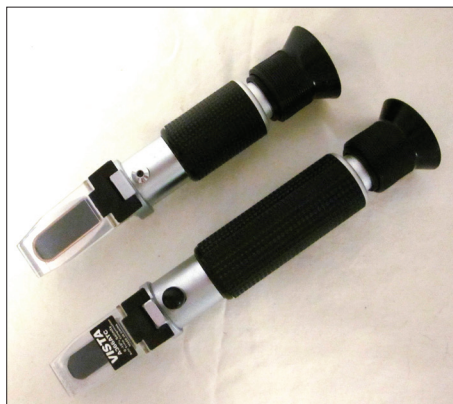
Photo 1: Brix (top) and salinity/specific gravity (bottom) refractometers. Photo courtesy of Dr. Robert Powitz.
