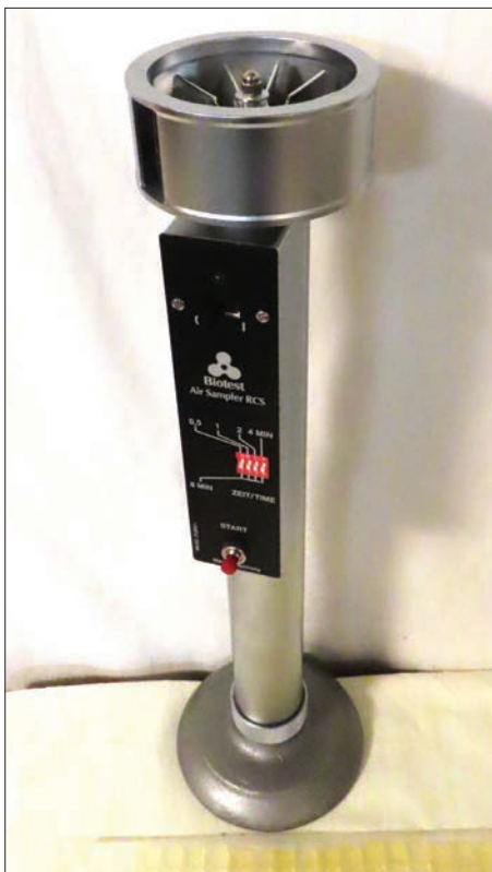
Photo 1. Centrifugal impactor sampler with agar sampling strip.
