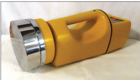
Photo 2. Sieve impactor sampler with a RODAC (replicate organism detection and counting) sampling head.
