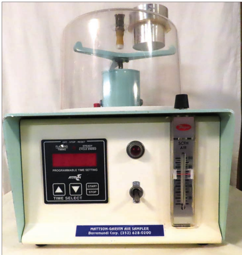
Photo 3. Slit-to-agar sampler with a clock mechanism.
