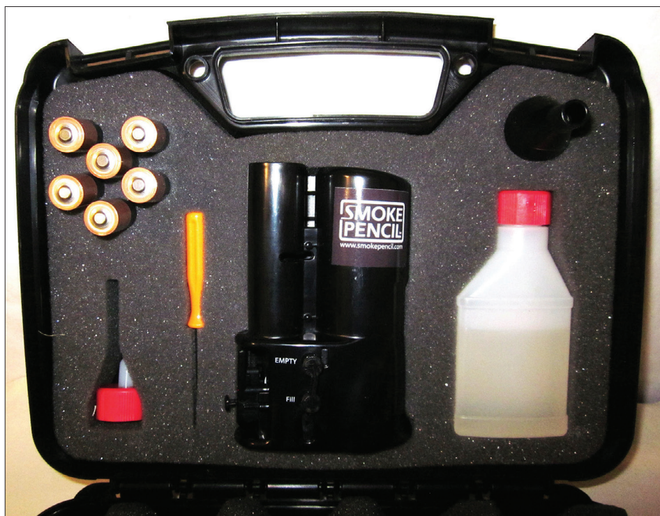
Photo 2: Example of a smoke pencil.
