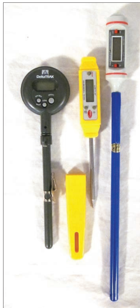
Photo 3: An example of three different thermistors. On the left is the "lollipop" thermistor thermometer, which replaced the maximum-registering liquid thermometer. In the center is a general-purpose pocket thermistor thermometer. On the right is a traceable digital thermistor thermometer with calibration.
