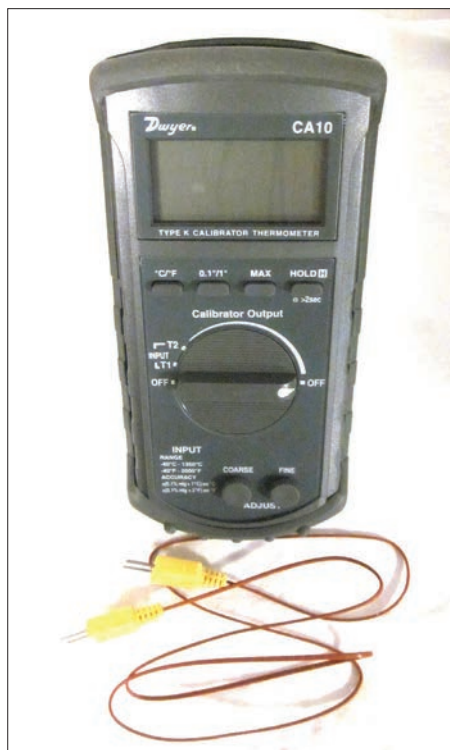
Photo 2: An example of a K-type wire thermocouple with a fixed-point calibration unit and male-male connectors used for calibration of both the thermocouple thermometer and K probes.
