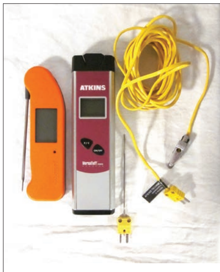
Photo 1: An example of two different types of thermocouples. On the left is a thermocouple with a tip-sensitive integrated probe. On the right is a thermocouple with a detachable needle K probe and an alligator clip K probe for measuring temperature in a commercial conveyor dishwasher.
