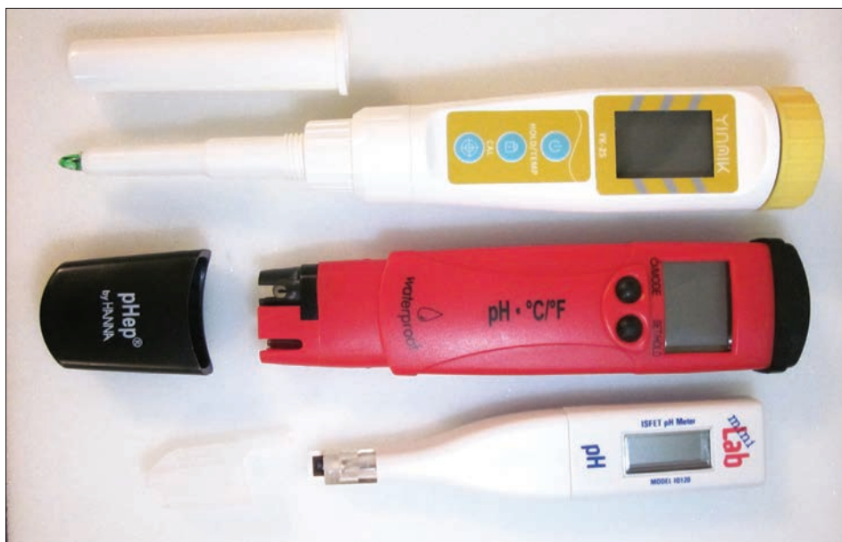
Different examples of portable pH instrumentation, including a high-accuracy single electrode (top), a double electrode (middle), and a single electrode pen (bottom). Photo courtesy of Dr. Robert Powitz.
