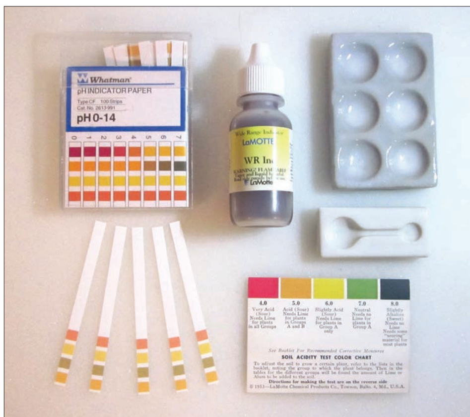
An example of pH indicator papers (1–14), along with pH indicator fluid, porcelain wells, and a color comparator. Photo courtesy of Dr. Robert Powitz.
