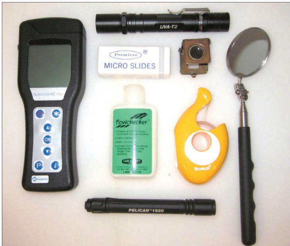
Photo 1. Basic field dust sampling tools. Outer circle: ATP luminometer and kit, UV flashlight, inspection mirror, and LED white light flashlight. Inner circle: Plain glass microscope slides, thread counter or linen tester, clear adhesive tape, and airflow detection powder. Photo courtesy of Dr. Robert Powitz.
